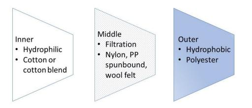
Figure 1. Non-medical mask construction using breathable fabrics such as cotton, cotton blends, polyesters, nylon and polypropylene spunbond that are breathable may impart adequate filtration performance when layered. Single- or double-layer combinations of advanced materials may be used if they meet performance requirements [85]
