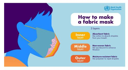
Although a minimum of three layers is recommended for non-medical masks for the most common fabric used, single, double or other layered combinations of advanced materials may be used if they meet performance requirements.
