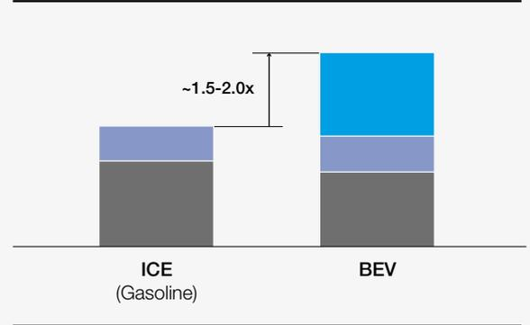
1.5-2.0x higher material emissions for BEV vs. ICEV due to energy-intensive battery production
