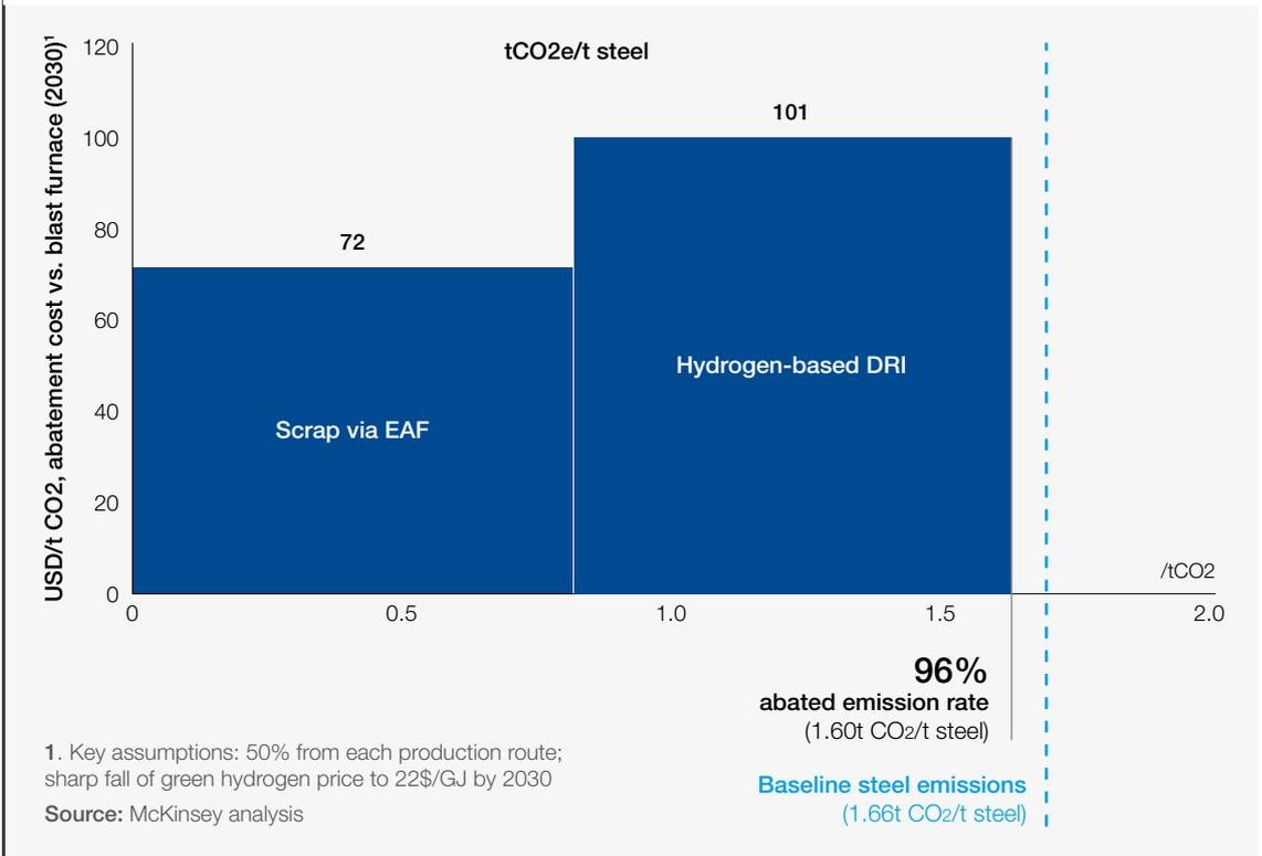
“ The levelized costs of hydrogen-based steelmaking would result in \$420–450/t steel, which may make this pathway more plausible than the (less technologically developed and economically feasible) CCS route.
