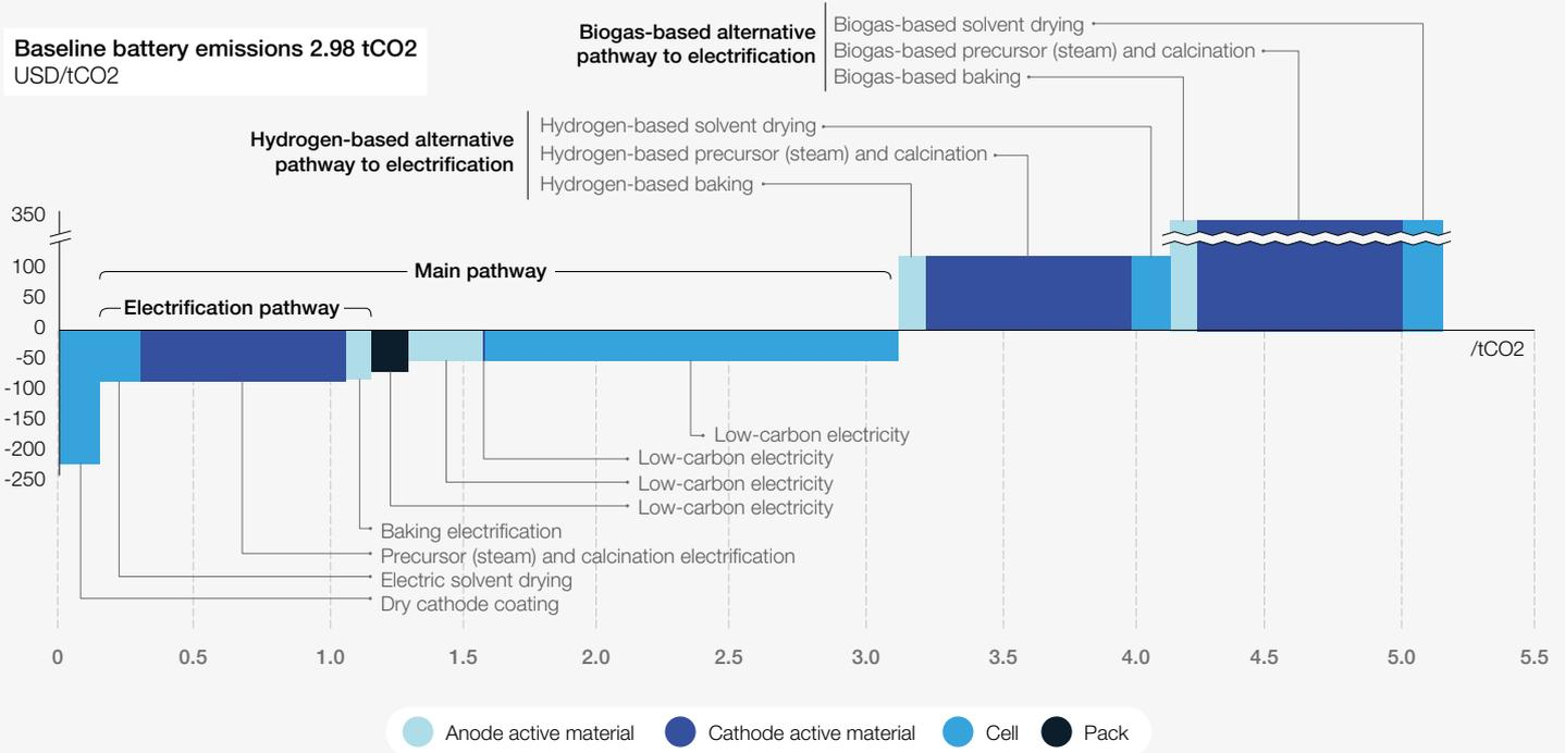
In this analysis a 92kWh battery per vehicle is considered, and only direct and indirect process emissions from fuels and electricity in the modelled production steps are included (mining or transport excluded)
