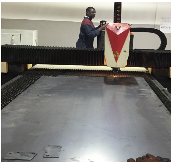
Use of CNC auto-cut laser machines for puncturing holes with specific dimensions in metal plates.
