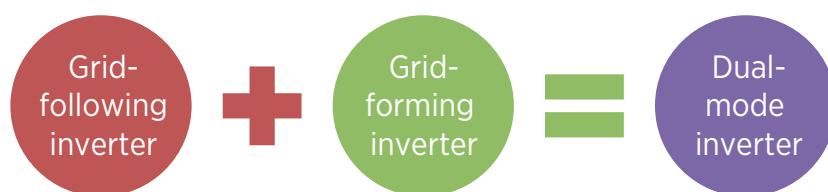
Figure 5: Relationship between grid-following, grid-forming and dual-mode inverters
