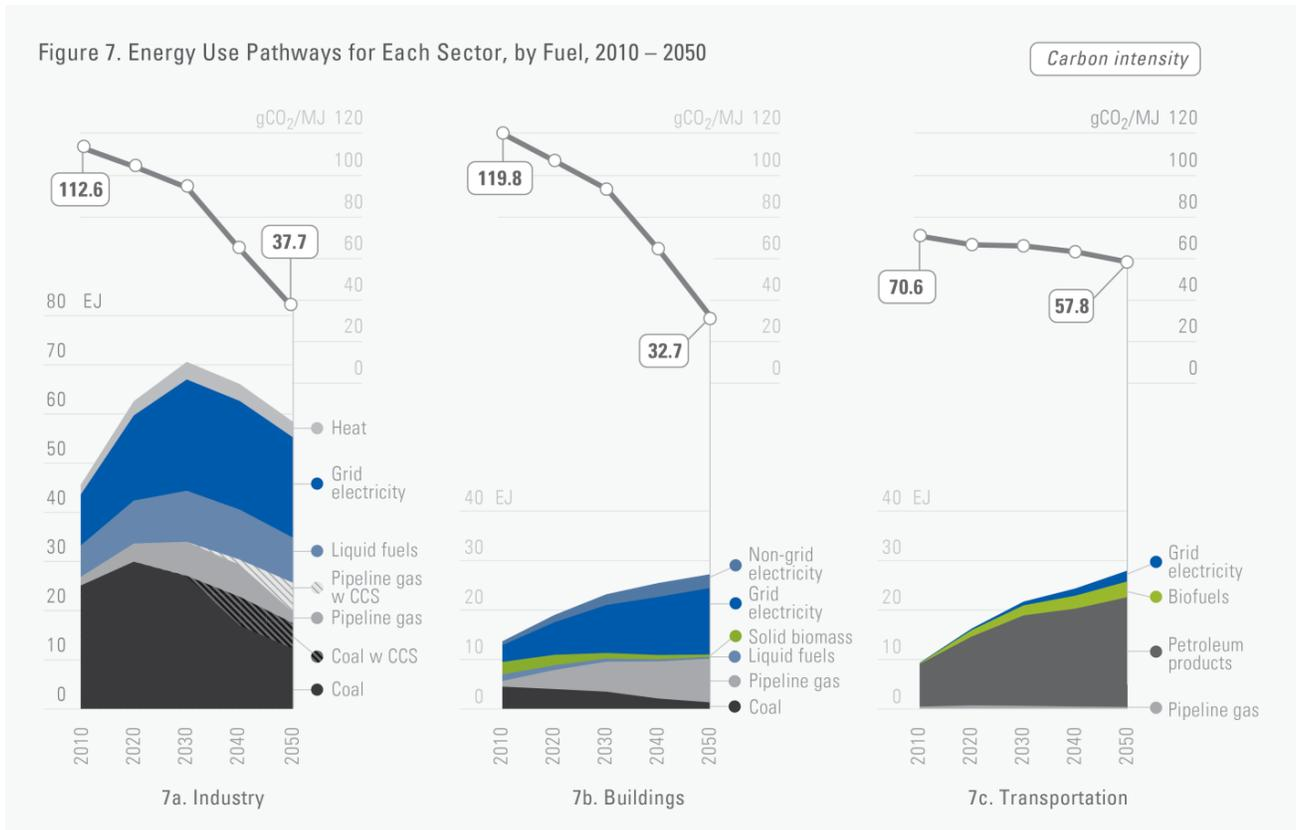
Note: Carbon intensity shown in Figure 7 for each sector includes both direct end-use emissions and indirect emissions related to electricity production.
