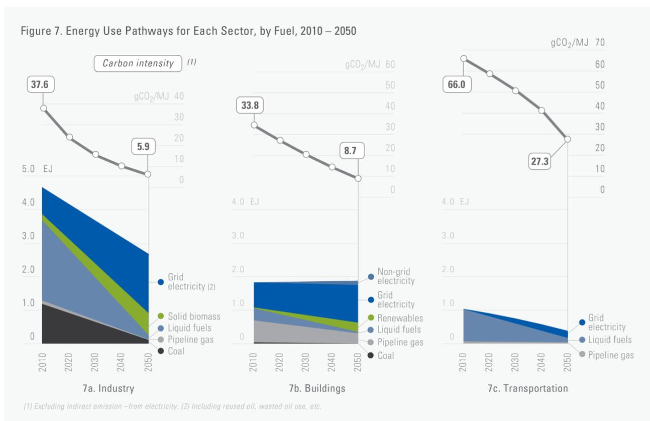
Note: Carbon intensity shown in Figure 7 for each sector includes only direct end-use emissions and excludes indirect emissions related to electricity or hydrogen production.
