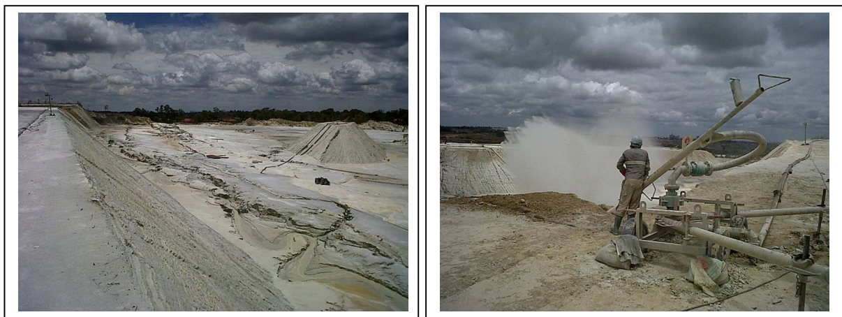
Photo 1(a) (left). The remnants of TDF 1L 8 after hydraulic mining. Photo 1(b) (right). Hydraulic cannon used to cut the tailings pile in the Cams TDF Cluster.
