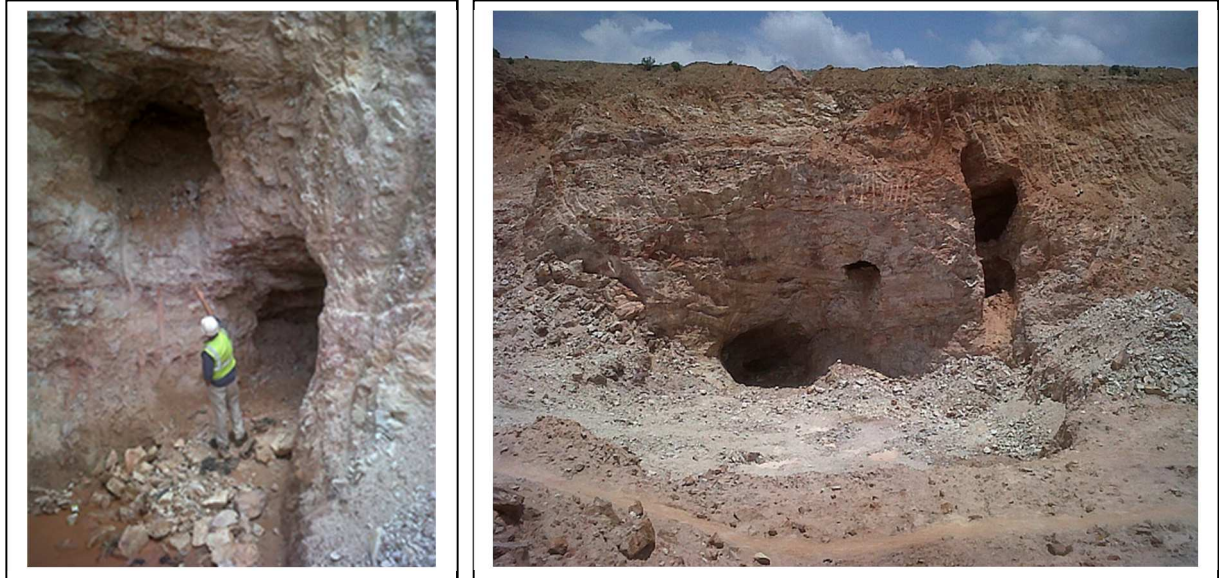
Photo 3(a) (left). A shallow underground working exposed through Closure Mining. Photo 3(b) (right). A typical cross section of an entry point into the void used by artisanal miners. The gold bearing reef targeted by these miners is visible as a grey band running parallel to the lower haulage that has been exposed.
