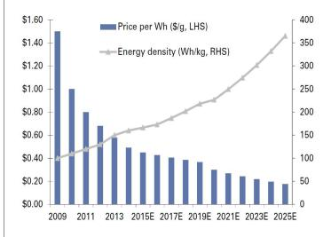
Most drones employ some form of lithium-ion technology, given they are small and lightweight. The batteries are well-suited for flights but have room to improve. Estimates show that these batteries will continue to increase in density (enabling longer, more efficient flights) and will decline in cost (Figure 6). This further demonstrates the growing opportunity for drones.
