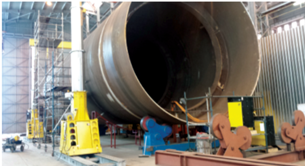
Figure 27: Fabrication of moulded LPG bullets (vessels) on Sunrise site
